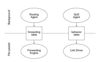
Packet forwarding is a simple task, performed on a per-packet basis as quickly as possible. It uses the packet header to find an entry in a routing table that determines the packet's output interface. Has changed little from the start.
