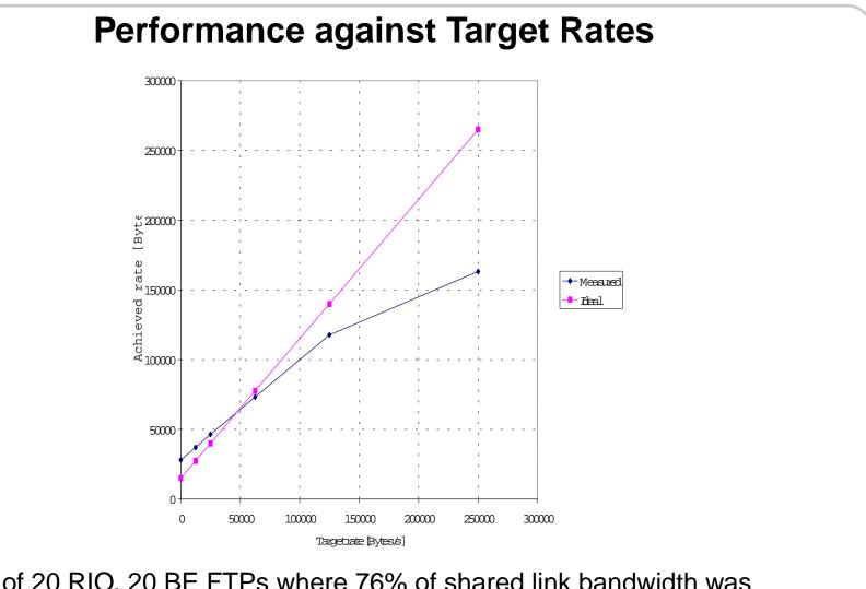
Mix of 20 RIO, 20 BE FTPs where 76% of shared link bandwidth was allocated to "ins". Five target rates were allocated to sets of four hosts each. The rates were: 0.1, 0.2, 0.5, 1.0, and 5.0 Mbps.
