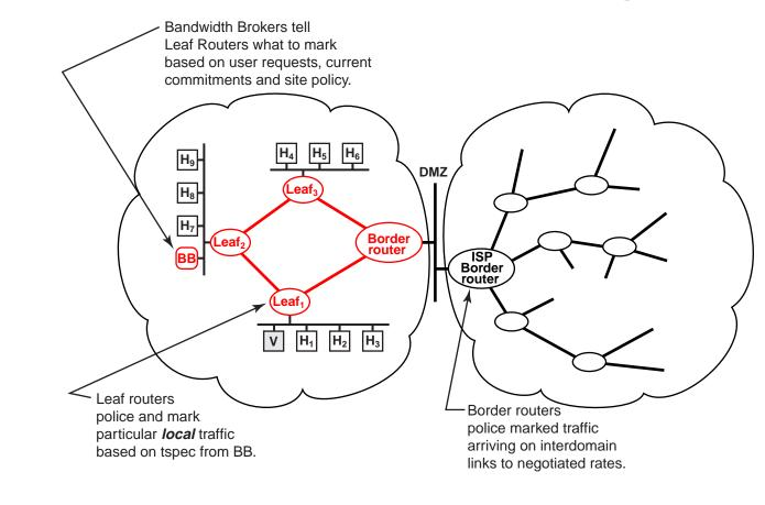
In a static or configured implementation, BB configures leaf/ edges with soft state information (COPS-PR?)
