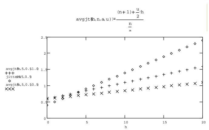
Using the average wait of half an MTU makes a larger difference than varying the link utilization, but both give some feel for what conditions have to occur to have jitter exceed one MTU at rate
